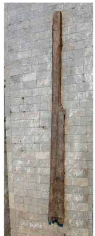
Plate 22.8 (left) Drawing of 11.07m long rudderpost comparison with a man; (right) Wood rudderpost. Length 10.06m. Nanjing Treasure Shipyard Relic Site Park
