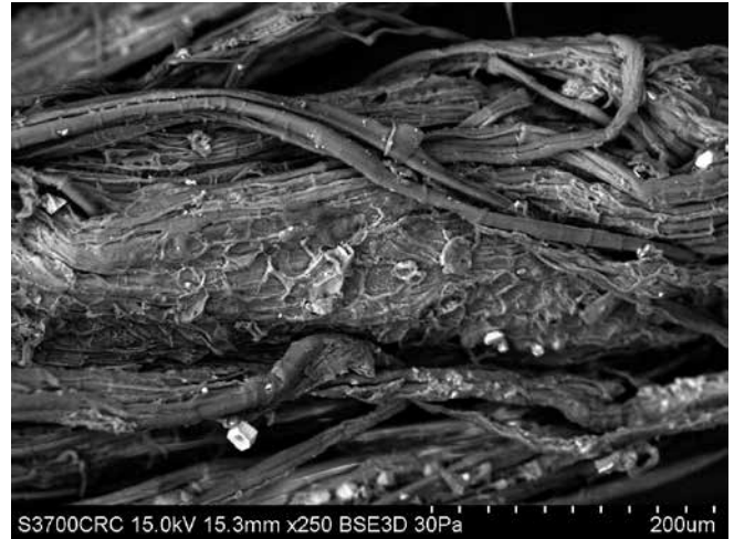
Plate 19.7 VP SEM image of Morus australis (Chinese mulberry) fibres from Ming dynasty paper money. British Museum, London CIB, EA.260
